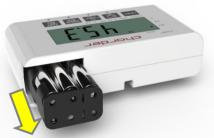
3. Place batteries in compartment (ensure polarity is correct)
