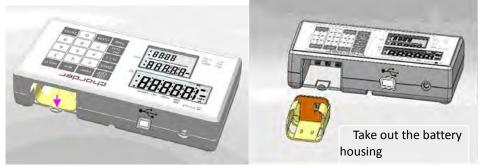
3. Use either rechargeable battery pack, or AA batteries
