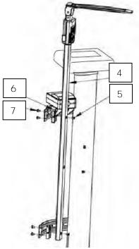
1. Attach brackets to column with round-head screws
