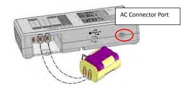
If **Lo** prompt displays on the LCD, please charge battery promptly to avoid battery damage.
