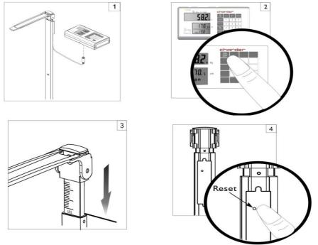
Slide measurement rod down completely. Turn on HM201D using **[BMI]** key on indicator. If height display is not at "120cm", press **[Reset]** key to calibrate to 120cm.
