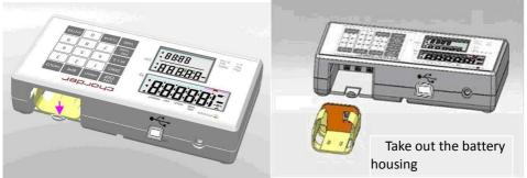
3. Use either rechargeable battery pack, or AA batteries
