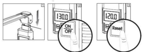
Slide measurement rod down completely. Turn on HM200D using **[ON/OFF]** key. If height display is not at "120cm", press **[Reset]** key to calibrate to 120cm.
