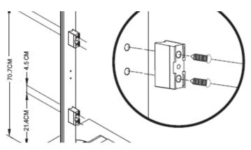
2. Attach height rod to fixing blocks using two screws.
