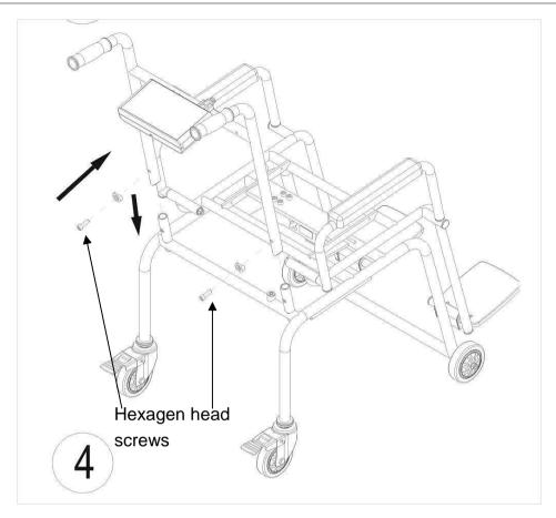
Assemble handle bar and fix with two hexagen socket head screws
