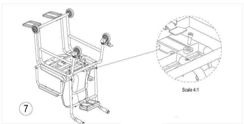
Assemble seat with screws.
